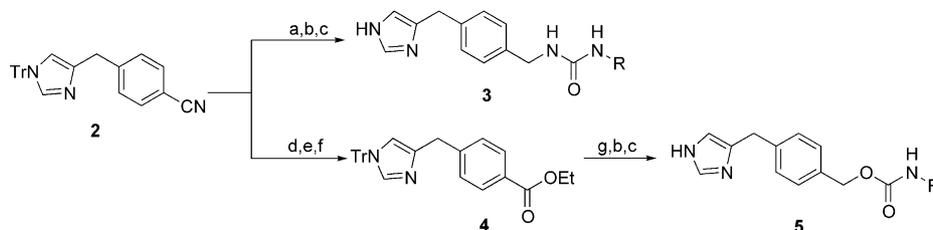
**Scheme 1.** Reagents and conditions: (a)  $H_2$ , Ra-Ni, MeOH/ $NH_3$ , 85%; (b) RNCO, pyridine; (c) 1 N HCl/MeOH; (d) 2 N NaOH, EtOH; (e)  $H_2SO_4$ , EtOH; (f) trityl chloride,  $Et_3N$ , 57% for steps d, e, and f; (g) DIBAL-H, THF, 94%. See Table 1 for the definition of R.
