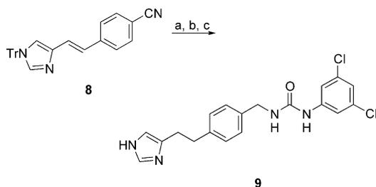
**Scheme 3.** (a)  $H_2$ , Ra-Ni,  $NH_3$ /MeOH; (b) 3,5- $Cl_2C_6H_4NCO$ ,  $CH_2Cl_2$ , 25% for two steps; (c) HCl/dioxane, 81%.
