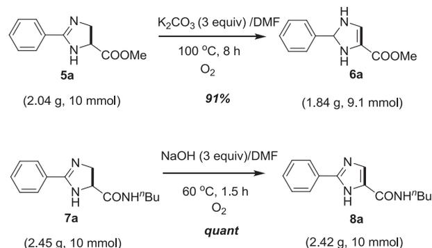
**Scheme 2.** The scalable oxidation of 2-imidazoline-5-carboxylates to 2-imidazoles by dioxygen.
