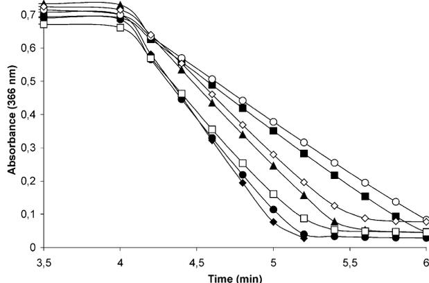
**Figure 3.** GSH Px-like activity of diselenides. Reactions were initiated by addition of 1.0 mM H<sub>2</sub>O<sub>2</sub> to the assay mixture containing 1.0 mM GSH, 0.26 mM NADPH, 1 U/mL GSSG reductase and 50 μM compound **4f** (◆), compound **4h** (●), compound **4j** (▲), compound **4i** (■), compound **4k** (○), compound **4b** (□) and compound **4e** (◇).
