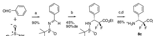
**Scheme 2.** General synthesis of  $\alpha,\alpha$ -difluoro-based inhibitors of SgTAM. Reagents: (a) CsCO<sub>3</sub>, DCM; (b) Zn<sup>0</sup>, ethyl bromodifluoroacetate, THF; (c) 6 N HCl; (d) *i*-PrOH, propylene oxide.
