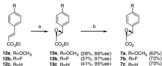
**Scheme 1.** Synthesis of epoxide-based inhibitors of SgTAM. Reagents: (a) 30 mol% Shi's epoxidation catalyst, oxone, NaHCO<sub>3</sub>, Na<sub>2</sub>EDTA, cat. TBAHS, H<sub>2</sub>O–CH<sub>3</sub>CN; (b) KOH, MeOH. Isolated yields and percent enantiomeric excess are indicated.
