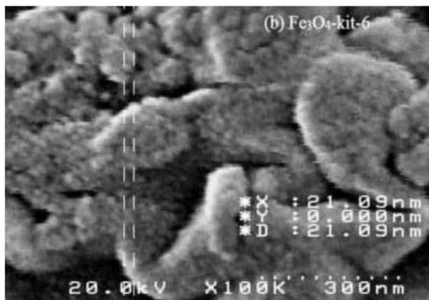
**Figure 1.** Scanning electron microscopy image of synthesized  $\text{Fe}_3\text{O}_4@SiO_2@KIT-6$ .
