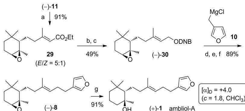
Scheme 4. Stereoselective synthesis of (1*S*,2*S*)-ambliol-A. Reagents and conditions: (a) (EtO)<sub>2</sub>POCH<sub>2</sub>CO<sub>2</sub>Et, NaH, THF; (b) DIBALH, THF, –40 °C; (c) 3,5-dinitrobenzoyl chloride, Py, DMAP cat.; (d) NaOH, MeOH, room temperature; (e) Ac<sub>2</sub>O, Py; (f) Li<sub>2</sub>CuCl<sub>4</sub> cat., THF, **10** 1.5 equiv., –20 °C to 0 °C; (g) LiEt<sub>3</sub>BH, THF, 0 °C then room temperature.
