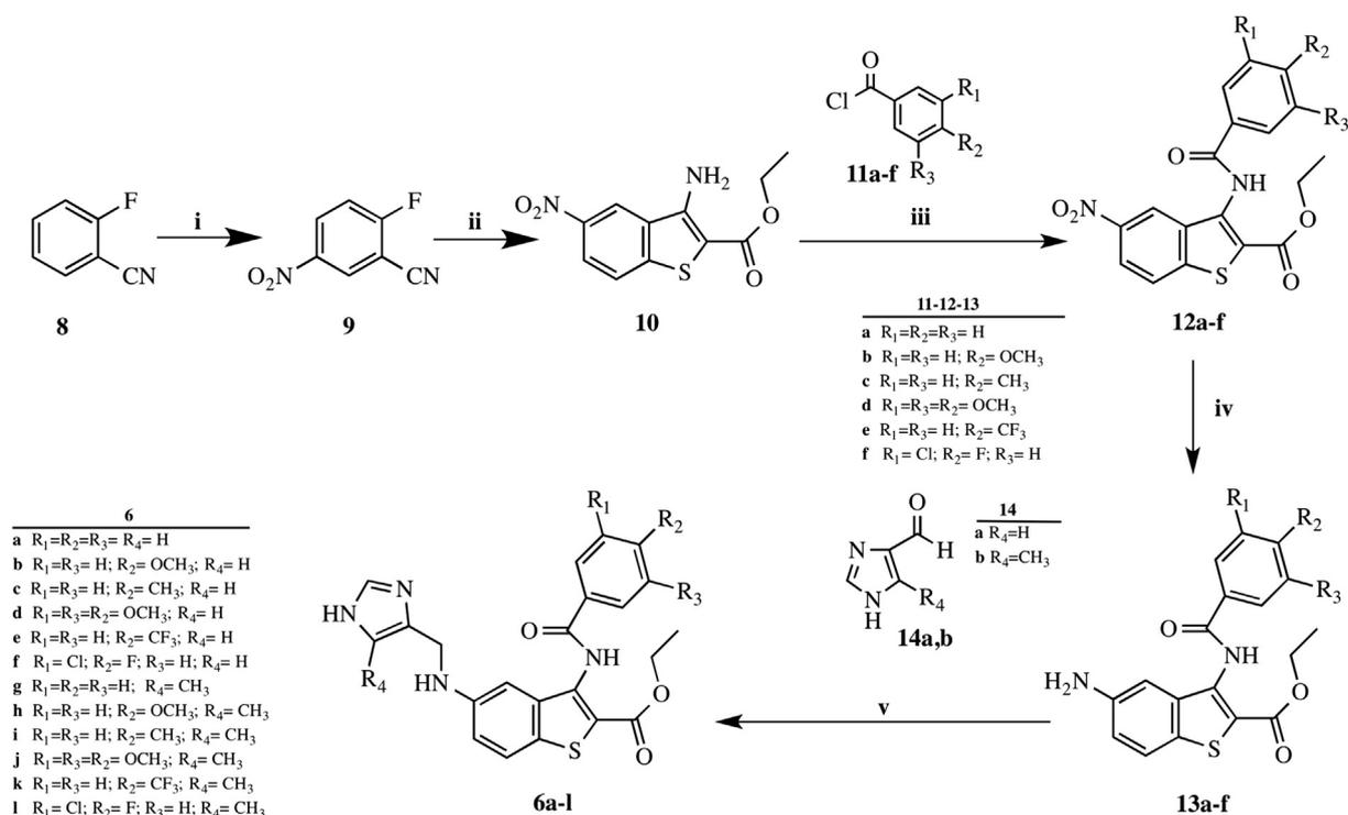
**Scheme 1.** Synthesis of ethyl 3-benzoylamino-5-[(1H-imidazol-4-yl-methyl)-amino]-benzo[b]thiophene-2-carboxylates **6a-l**. Reagents and conditions: (i): HNO<sub>3</sub>:H<sub>2</sub>SO<sub>4</sub> (1:1), N<sub>2</sub>, 0 °C, 2 h; (ii): ethyl thioglycolate/NaH 60%, anhydrous DMSO; (iii): pyridine, rt, 12 h; (iv): 10% Pd/C, H<sub>2</sub>, ethanol, rt 2 h; (v): NaCNBH<sub>3</sub>, ethanol/AcOH, 2 h.
