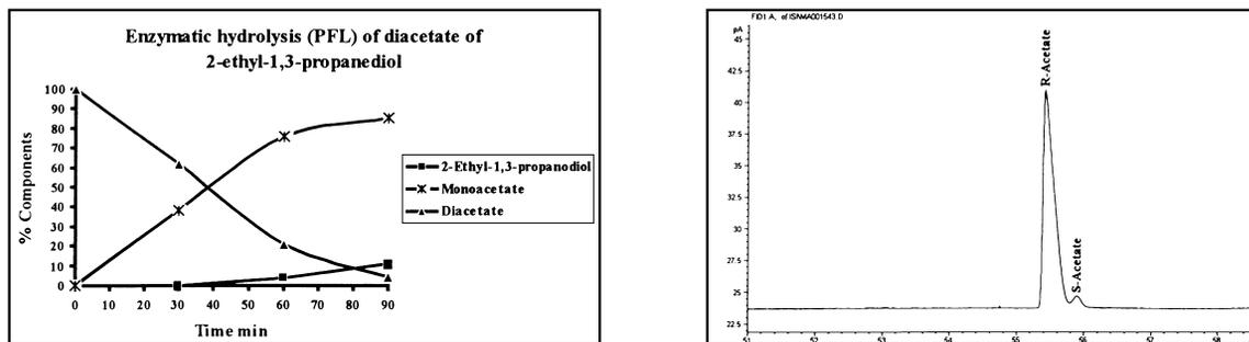
Figure 2. Kinetic data for enzymatically (PFL) catalyzed partial hydrolysis of **2** and GLC analysis (ee) on a  $\beta$ -DEX™ column
