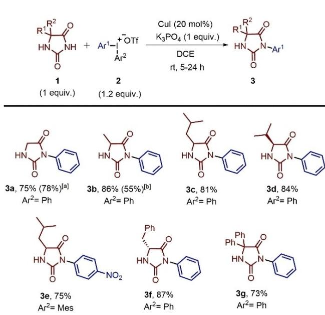
**Scheme 3.** Scope of Hydantoin. Reaction conditions: 3-aryl-5,5-dimethylhydantoin (0.25 mmol), iodonium salt (0.3 mmol), CuI (20 mol%) and K<sub>3</sub>PO<sub>4</sub> (0.25 mmol) in DCE (0.1 M). [a] 2 equiv. of 2a. [b] 2 equiv. of 1b. Isolated yields.
