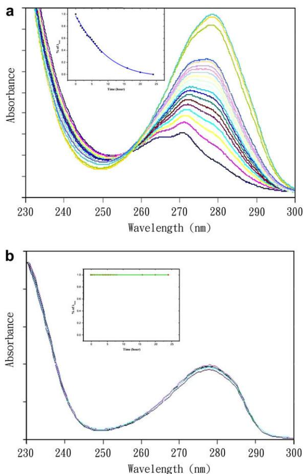
**Figure 2.** UV-visible spectra for indication of stability of NDGA derivatives (a) G<sub>4</sub>N (**4**) degradation in Milli-Q Water. (b) P<sub>4</sub>N (**5b**) present in Milli-Q Water after 28 days.
