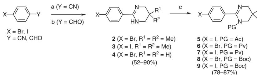
**Scheme 2** Reagents and conditions: (a) Y = CN: amine, TsOH, diethylene glycol, 100 °C; (b) Y = CHO: amine, NBS, CH<sub>2</sub>Cl<sub>2</sub>, 0 °C to r.t.; (c) acid anhydride, Et<sub>3</sub>N, CH<sub>2</sub>Cl<sub>2</sub>, 0 °C to r.t.
