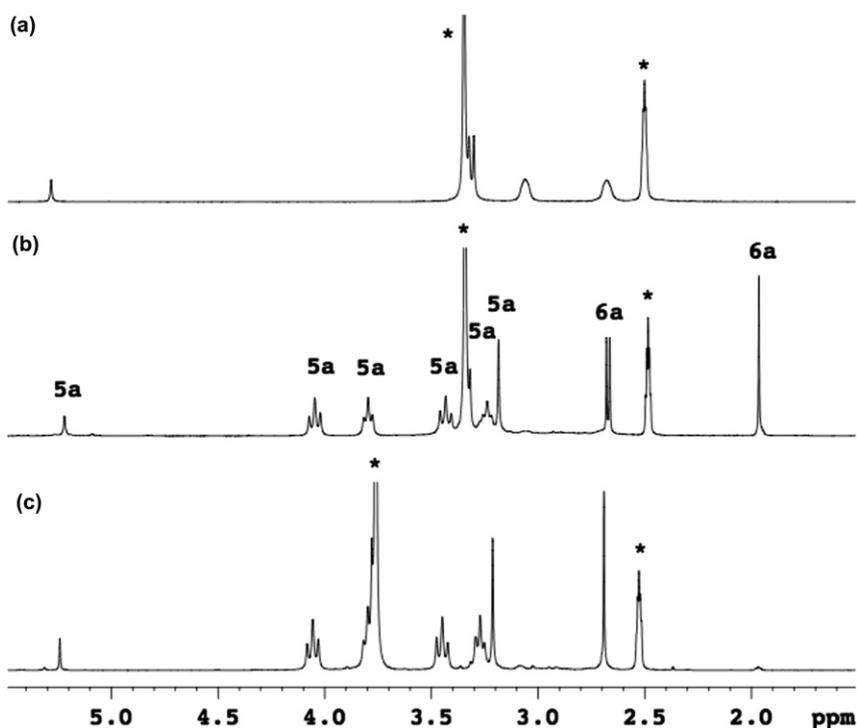
**Figure 2.** <sup>1</sup>H NMR spectra of (a) **4Aa**, (b) **4Aa** after reaction with 0.5 equiv of zinc perchlorate, (c) **4Aa** after reaction with 0.5 equiv of zinc perchlorate in the presence of D<sub>2</sub>O. Asterisk (\*) indicates signals of DMSO and H<sub>2</sub>O.
