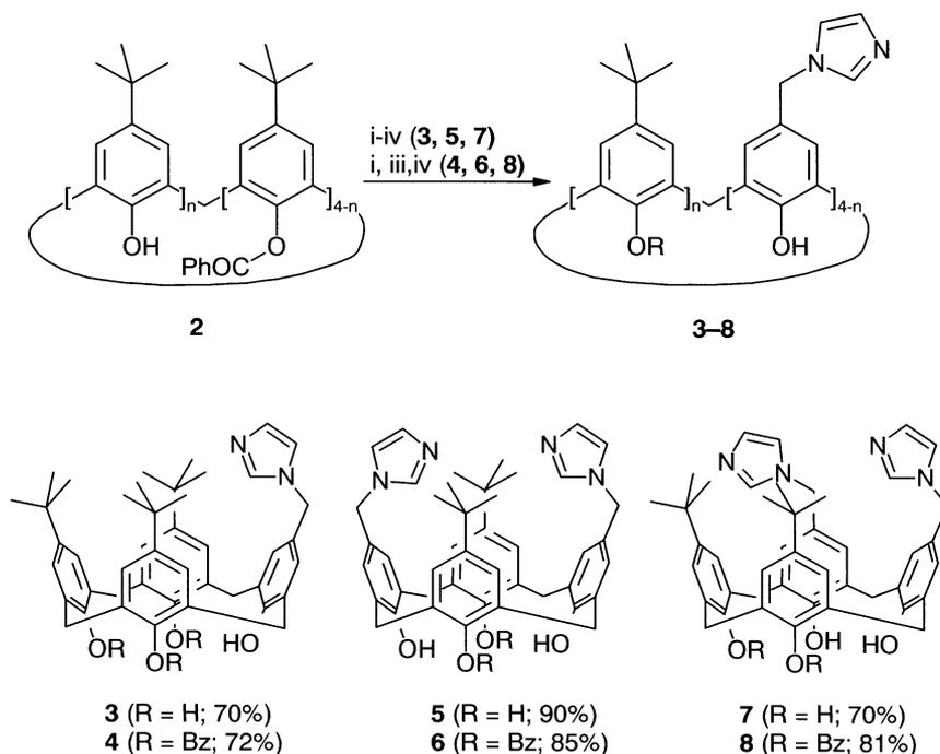
**Scheme 1.** Synthesis of calix[4]arenes **3–8**; (i)  $\text{AlCl}_3$ , toluene, rt, 69–98%; (ii)  $\text{EtOH}/\text{H}_2\text{O}$ ,  $\text{NaOH}$ , 3 days,  $80^\circ\text{C}$ , 94–98%; (iii)  $\text{CH}_2(\text{NMe}_2)_2$ ,  $\text{THF}/\text{HOAc}$ , 48 h, rt, 92–95%; (iv) 1.  $\text{MeI}$ ,  $\text{DMSO}$ , 1 h, rt; 2. imidazole, 3 h,  $80^\circ\text{C}$ , 70–90% ( $\text{R}=\text{H}$ ), 72–85% ( $\text{R}=\text{Bz}$ ).
