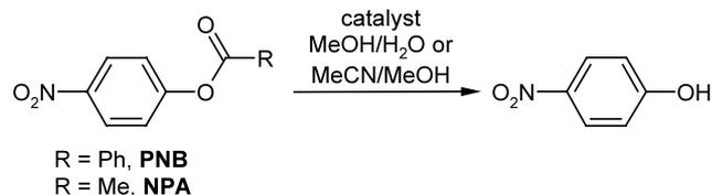
**Scheme 2.** Hydrolysis of *p*-nitrophenyl benzoate (**PNB**) and acetate (**PNA**) catalysed by macrocycles **3–8**.
