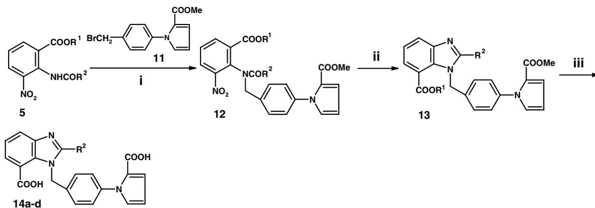
**Scheme 2.** Reagents and conditions: (i) NaH, DMF, rt (65–76%); (ii) Fe/HCl, MeOH, reflux (80–88%); (iii) NaOH, MeOH/H<sub>2</sub>O, reflux; then HCl, rt (59–71%).
