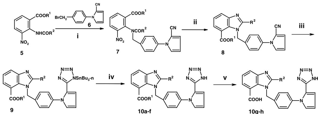
**Scheme 1.** Reagents and conditions: (i) NaH, DMF, rt (69–78%); (ii) Fe/HCl, MeOH, reflux (75–84%); (iii) *n*-Bu<sub>3</sub>SnCl, NaN<sub>3</sub>, toluene, reflux; (iv) HCl, MeOH, rt (38–55%); (v) LiOH, THF/H<sub>2</sub>O, 80 °C, then HCl, rt (40–42%).
