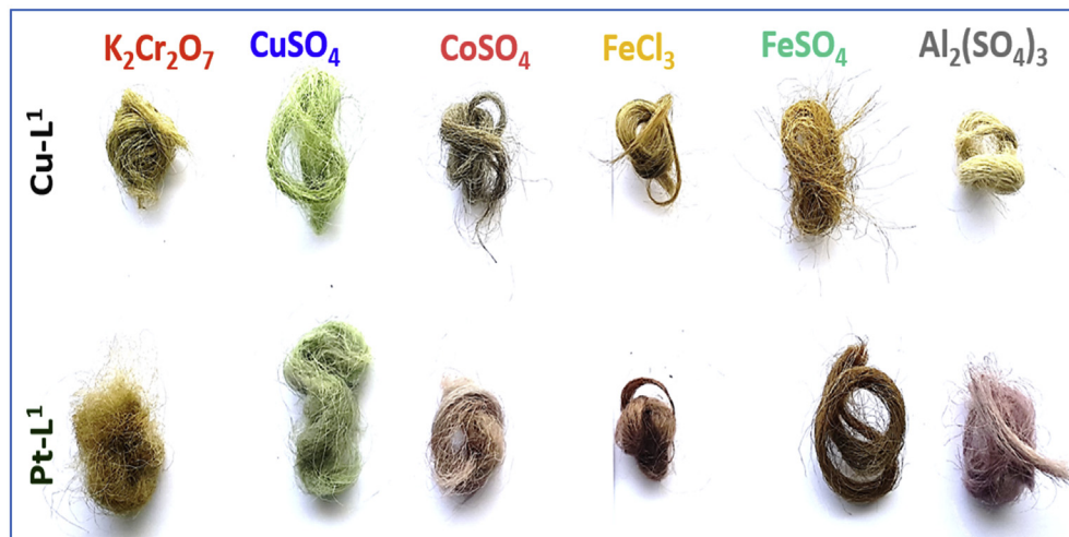
Fig. 9. a, b) Dyeing of wool with the disperse black 9, HL 1 , [Cu(L 1 )Cl(H 2 O)]3H 2 O and [Pt(L 1 )Cl(H 2 O) 2 ]2H 2 O in water.
