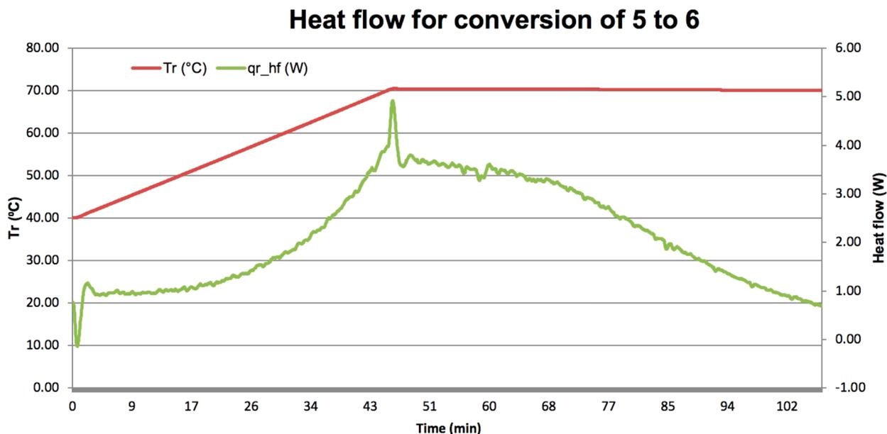
Figure 7. Heat flow for the conversion of intermediate 5 to product 6.
