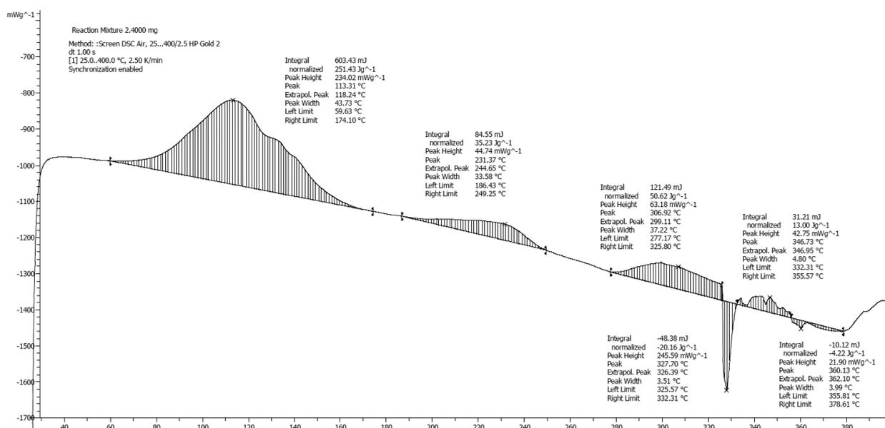
Figure 8. DSC curve of the reaction mixture
