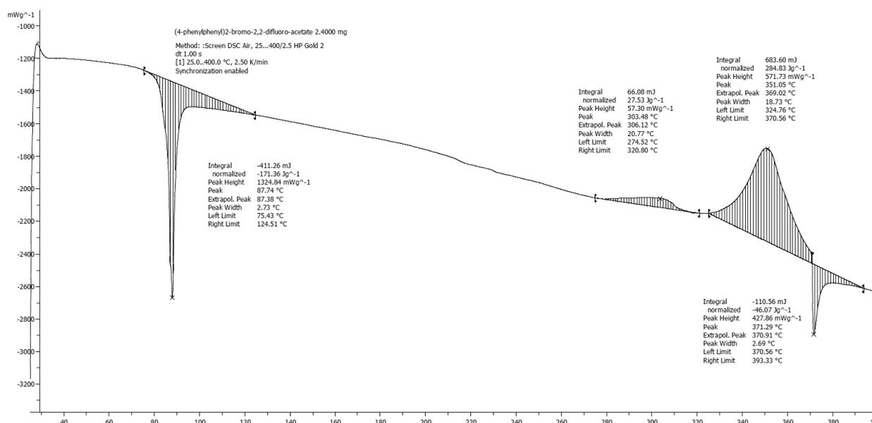
Figure 5. DSC curve (range: 25–400 °C) of BBDFFA.
