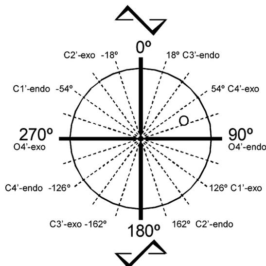
**Figure 2.** Graphical representation of the pseudorotational cycle,<sup>48</sup> which defines all of the possible ribose ring conformations. The phase angle of pseudorotation ( $P$ ) describes the geometry of the ribose puckering. The (N)-methanocarba ring system adopts a C2'-exo conformation, and the (S)-methanocarba ring system adopts a C3'-exo conformation. The 2-OBH ring system maintains a C1'-exo conformation, in the (S)-region.
