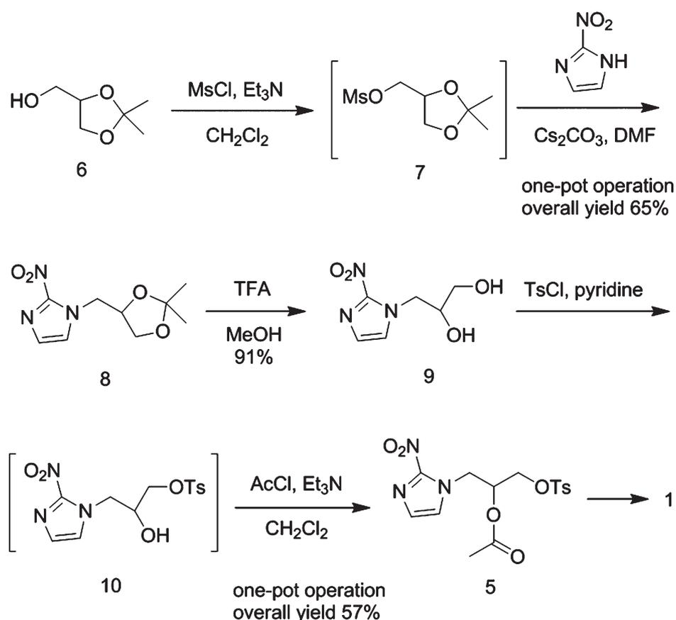
**Scheme 2.** Synthesis of [ $^{18}\text{F}$ ]-FMISO precursor from (2,2-dimethyl-1,3-dioxolan-4-yl)methanol (method B).
