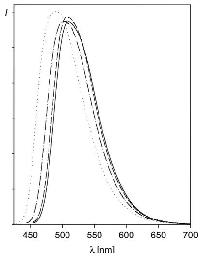
**Figure 4.** Comparison of fluorescence emission band in chloroform of *N,N'*-carbonyl-bridged dipyrinones substituted at C(3) with: *n*-decyl (dotted line), phenyl (dash-dotted line), *p*-ethoxytetrafluorophenyl (dashed line), and pentafluorophenyl (solid line). The vertical axis plots relative intensity (*I*) of fluorescence emission.
