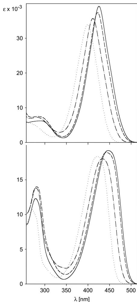
**Figure 3.** Comparison of UV-vis spectra in chloroform of dipyrinones (upper panel) and their *N,N'*-carbonyl-bridged derivatives (lower panel) substituted at C(3) with: *n*-decyl (dotted line), phenyl (dash-dotted line), *p*-ethoxytetrafluorophenyl (dashed line), and pentafluorophenyl (solid line).
