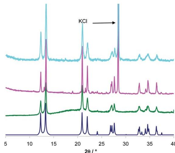
**Fig. 12** Diffraction patterns for  $[\text{Zn}(\text{pz})_2]_n$  **9**. Blue = calculated from MAPCOV;<sup>15</sup> green =  $3\text{Zn}(\text{OH})_2 \cdot 2\text{ZnCO}_3 + 10\text{Hpz}$ ; pink = **4** + 2KOH; turquoise = **4** + 2t-BuOK.
