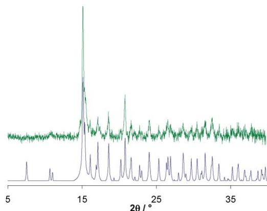
**Fig. 14** Powder diffraction patterns for [Co(im)<sub>2</sub>]<sub>n</sub> (**14**). Blue = calculated from IMZYCO01; green = [Co(Him)<sub>2</sub>Cl<sub>2</sub>] + 2KOH.
