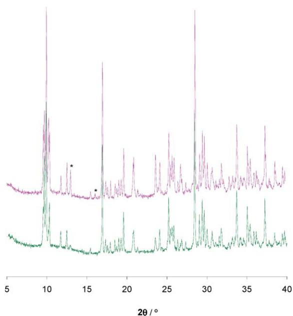
Fig. 5 XRPD patterns for samples of  $[H_2pz]_2[CuCl_4]$  **5**. Green = mechanochemical synthesis; pink = from HCl gas absorption. \* = peaks from **6**.
