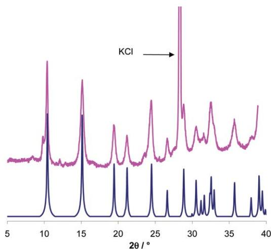
**Fig. 10** XRPD patterns for  $[\text{Cu}(\text{pz})_2]_n$  (**8**) + 2KCl. Blue = calculated from the crystal structure NAPBIQ;<sup>16</sup> pink = product of grinding **6** + 2KOH.
