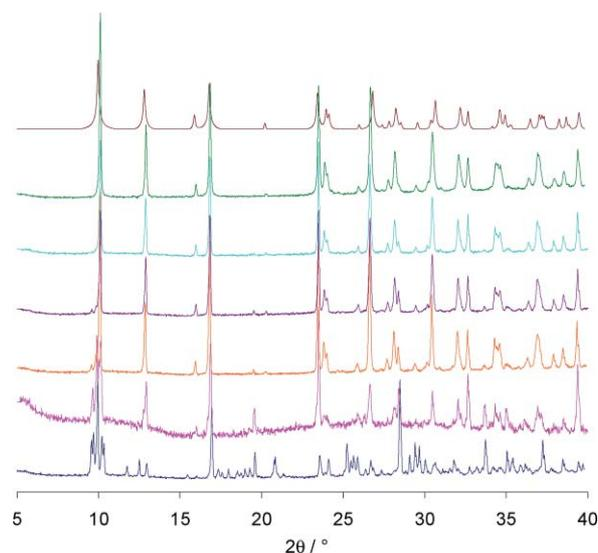
Fig. 6 XRPD patterns for the loss of HCl from  $[H_2pz]_2[CuCl_4]$  **5**. Blue = 0 h; pink = 24 h; orange = 48 h; turquoise = 96 h; green = **6** (mechanochemical synthesis); brown = calculated from the crystal structure.
