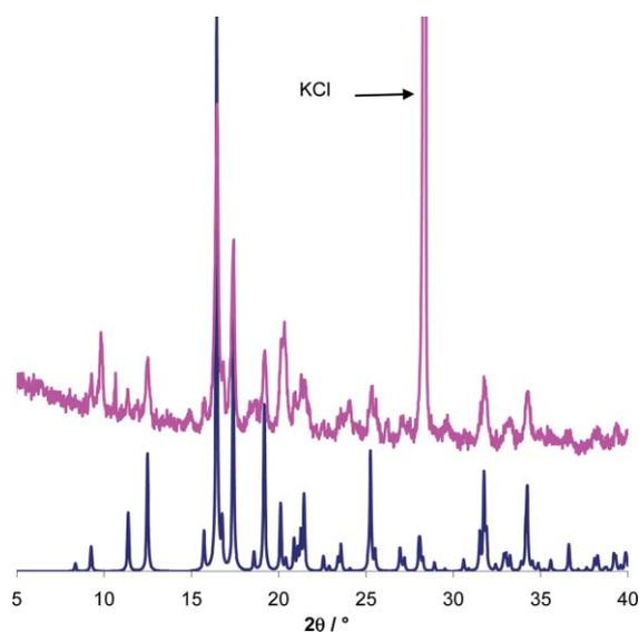
**Fig. 13** Powder diffraction patterns for [Cu(im)<sub>2</sub>]<sub>n</sub> (G-12). Blue = calculated from CUIMDZ02; pink = [CuCl<sub>2</sub>(Him)<sub>2</sub>] + 2KOH.
