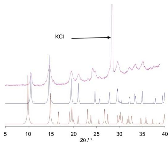
Fig. 9 XRPD patterns for **7**. Brown and blue = calculated from the single crystal structures of  $\beta$ - $[\text{Ni}(\text{pz})_2]_n$  and  $\alpha$ - $[\text{Ni}(\text{pz})_2]_n$  respectively; pink = mechanochemical reaction of  $[\text{NiCl}_2(\text{Hpz})_2] + 2\text{KOH}$ .
