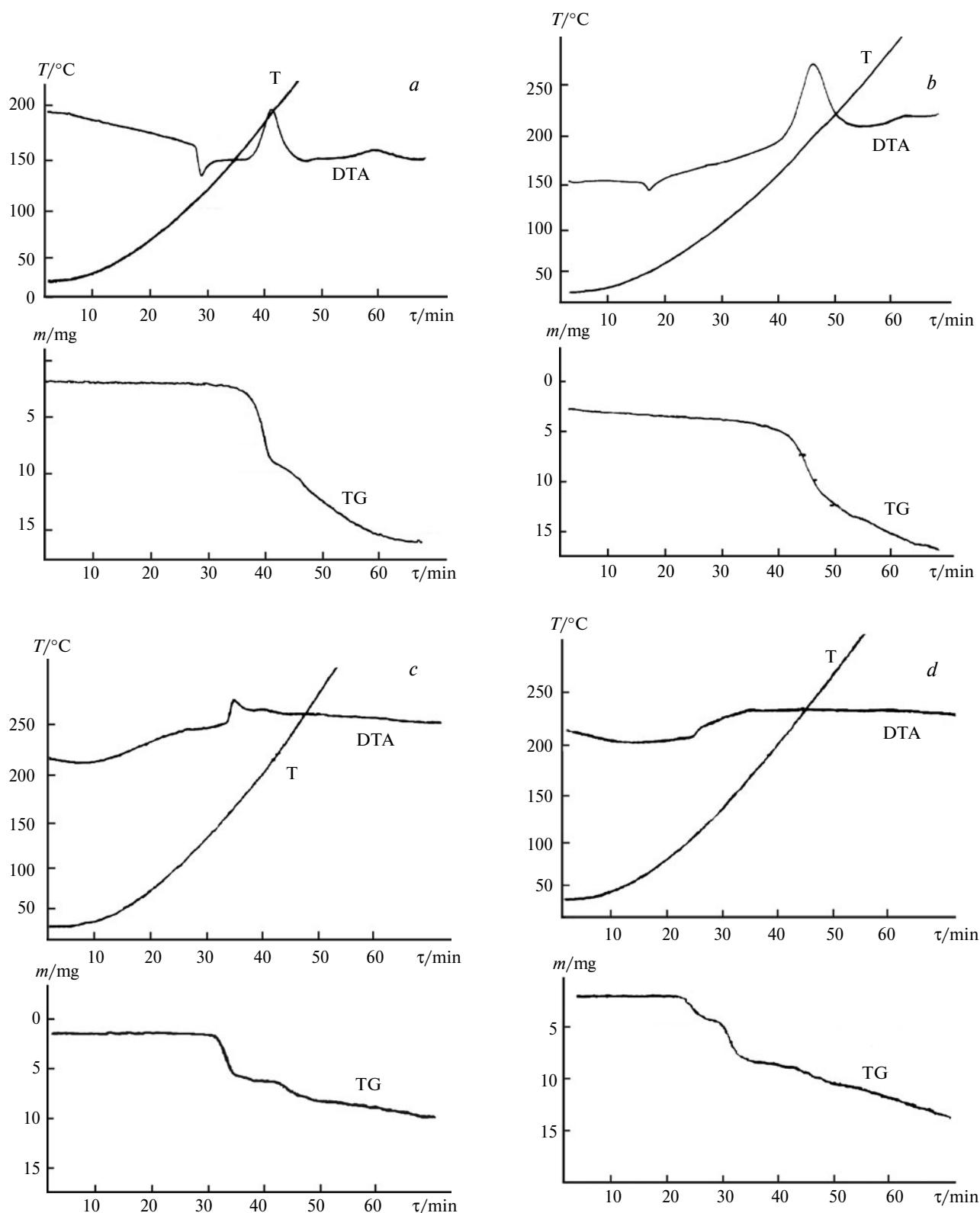
**Fig. 1.** Thermogravimetric (TG), temperature (T), and thermal differential (DTA) curves of (3-nitro-1*H*-1,2,4-triazol-1-yl)methyl nitrate (**3**) (*a*), 1-(azidomethyl)-3-nitro-1*H*-1,2,4-triazole (**5**) (*b*), 5,5'-dinitro-2,2'-di(nitroxymethyl)-2*H*,2'*H*-3,3'-bi(1,2,4-triazole) (**8a**) (*c*), 5,5'-dinitro-2,2'-di(nitroxymethyl)-2*H*,2'*H*-3,3'-(nitromethylene)bis(1*H*-1,2,4-triazole) (**9**) (*d*).
