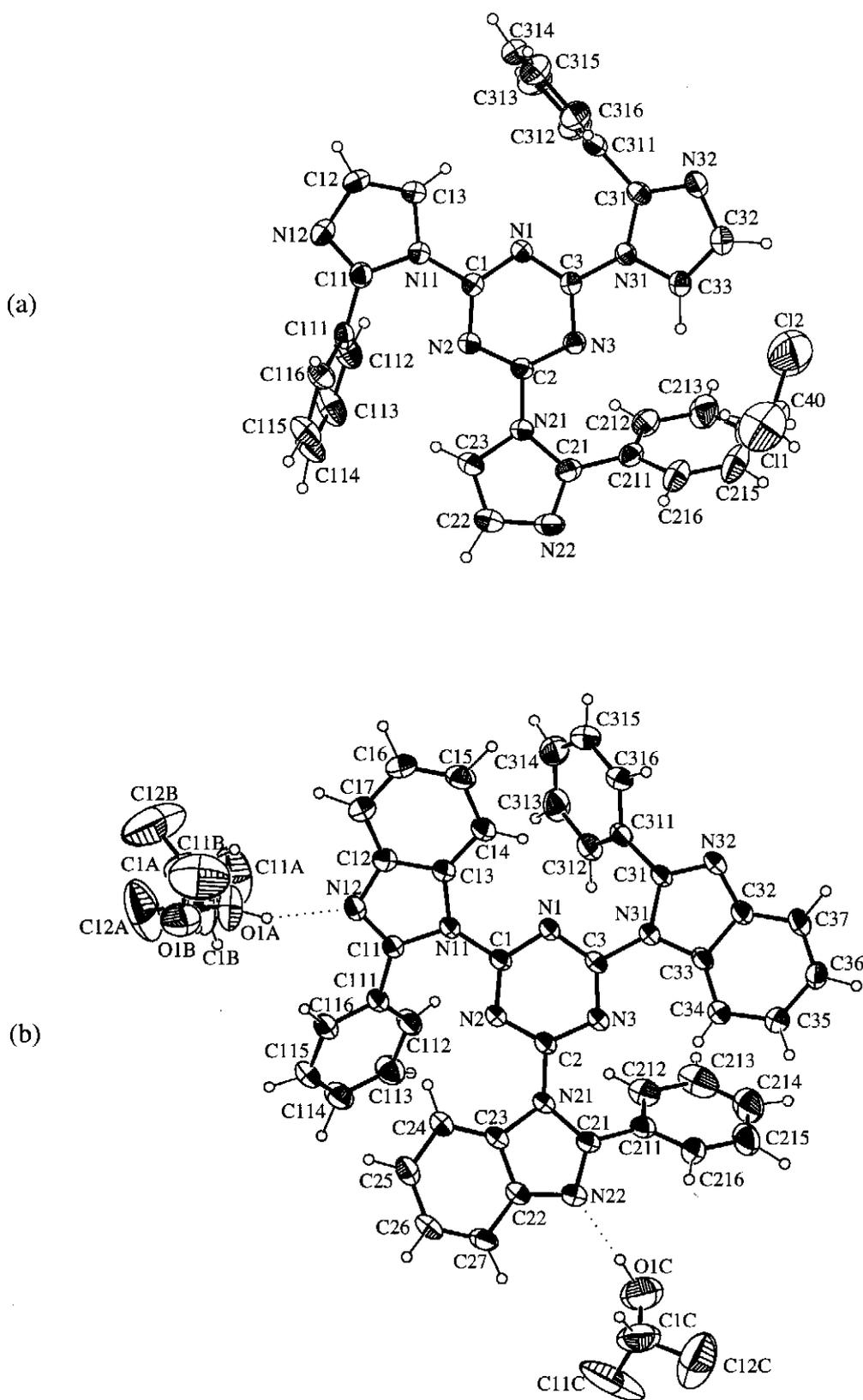
**Figure 1.** Molecular structure and atomic numbering of the triazine derivatives: (a) **6c** and (b) **8c**. Displacement ellipsoids are scaled to enclose 30% probability, and the hydrogen atoms are denoted as spheres of 0.1 Å radii.
