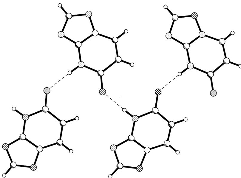
Fig. 2. Hydrogen-bonded chain along the  $\langle 011 \rangle$  direction in the crystal structure of 5HtpO.
