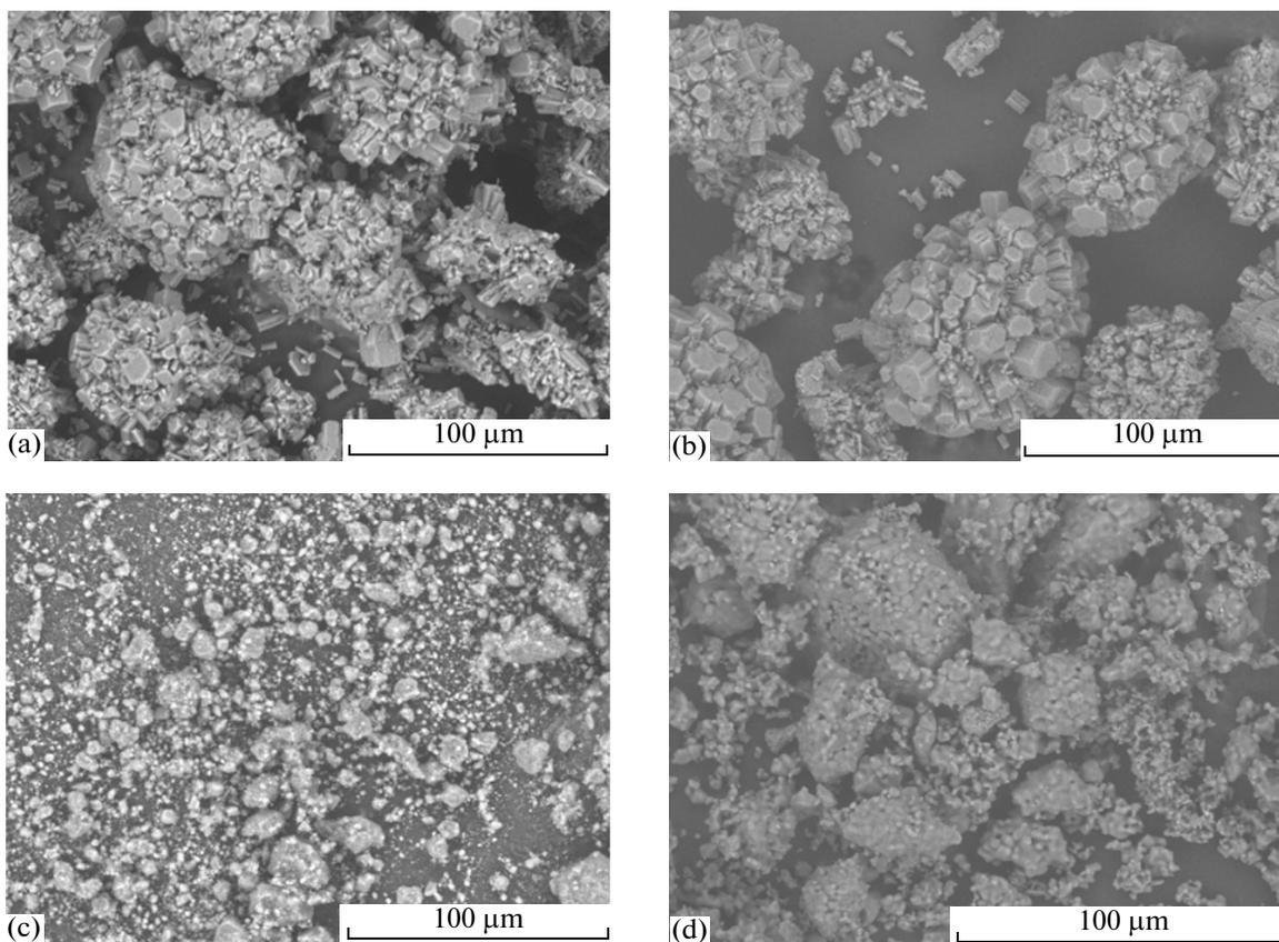
**Fig. 6.** Electron microscopic micrographs of the (a) unactivated aluminum hydroxide, (b) the product of its reaction with lithium carbonate, (c) aluminum hydroxide mechanically activated for 10 min, and (d) the product of the reaction of the mechanically activated aluminum hydroxide with lithium carbonate.
