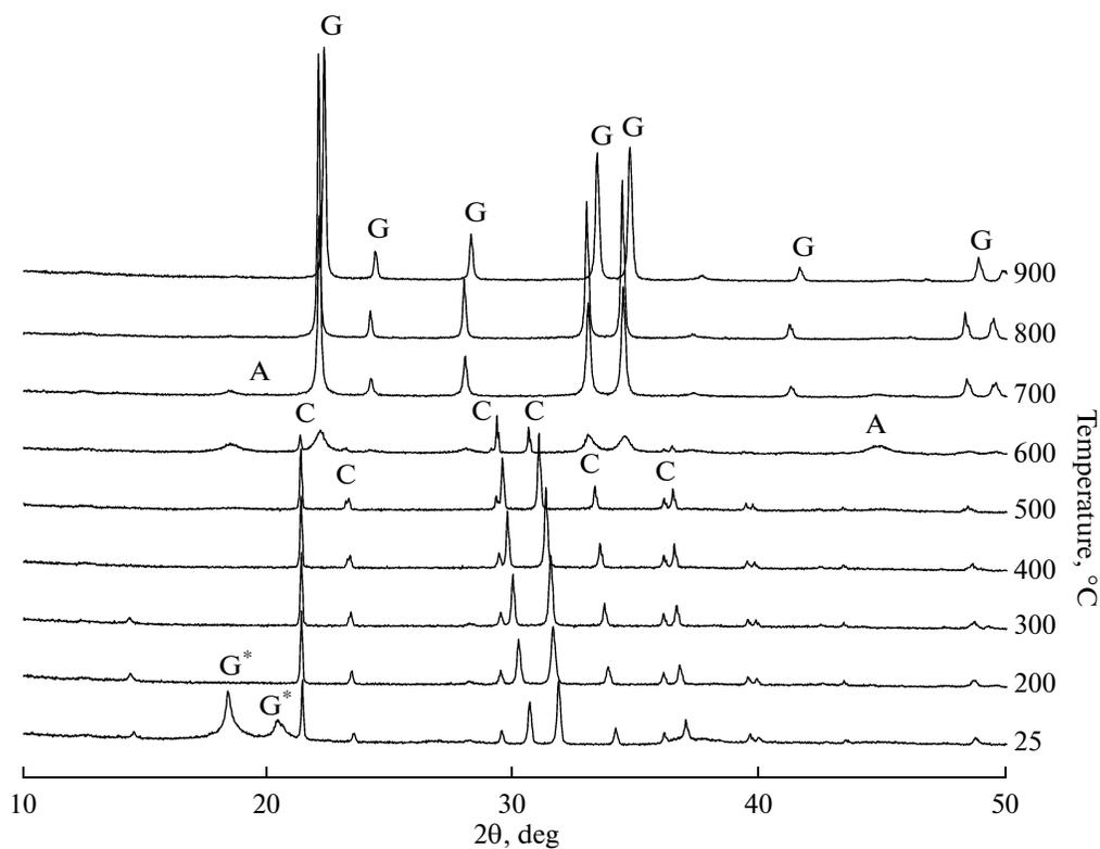
**Fig. 3.** In situ XRD patterns of a mixture of aluminum hydroxide mechanically activated for 5 min and lithium carbonate. A =  $\alpha$ - $\text{LiAlO}_2$ , G =  $\gamma$ - $\text{LiAlO}_2$ , B = boehmite,  $G^*$  =  $\text{Al}(\text{OH})_3$ , C =  $\text{Li}_2\text{CO}_3$ .
