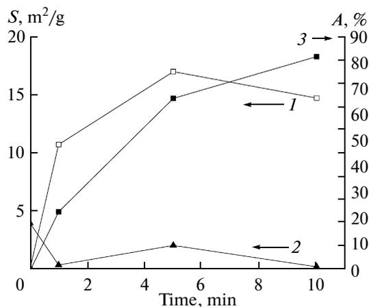
**Fig. 5.** (1) Specific surface of aluminum hydroxide, (2) specific surface of lithium aluminate, and (3) amorphous phase content of mechanically activated aluminum hydroxide as functions of milling time (the percentage of the X-ray amorphous phase was evaluated from the integrated intensity of the reflection at  $d/n = 4.82 \text{ \AA}$ ).
