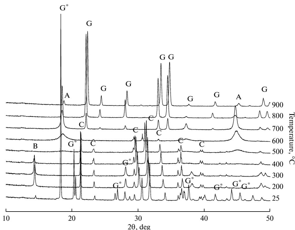
**Fig. 2.** In situ XRD patterns of a mixture of lithium carbonate and unactivated aluminum hydroxide. A =  $\alpha$ -LiAlO<sub>2</sub>, G =  $\gamma$ -LiAlO<sub>2</sub>, B = boehmite, G\* = Al(OH)<sub>3</sub>, C = Li<sub>2</sub>CO<sub>3</sub>.
