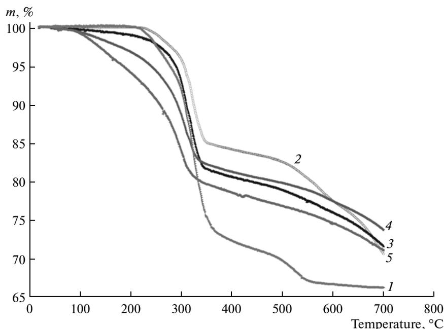
**Fig. 1.** Weight loss curves of (1) gibbsite, (2) a mixture of gibbsite and lithium carbonate, and (3–5) mixtures of lithium carbonate and mechanically activated aluminum hydroxide. Milling time of (3) 1, (4) 5, and (5) 10 min; sample weight, 200 mg; heating at a rate of  $10^\circ\text{C}/\text{min}$  in air.
