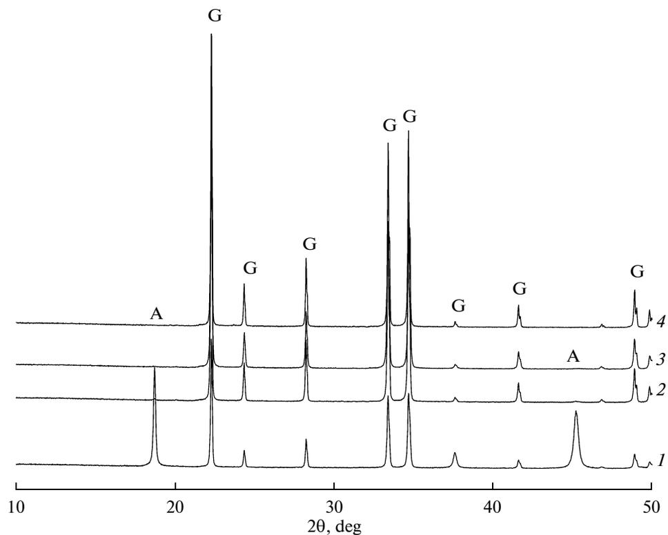
**Fig. 4.** XRD patterns taken after heat treatment (800°C, 4 h) of a mixture of  $\text{Al}(\text{OH})_3$  mechanically activated for (2) 1, (3) 5, and (4) 10 min and  $\text{Li}_2\text{CO}_3$ ; (1) without MA. A =  $\alpha$ - $\text{LiAlO}_2$ , G =  $\gamma$ - $\text{LiAlO}_2$ .
