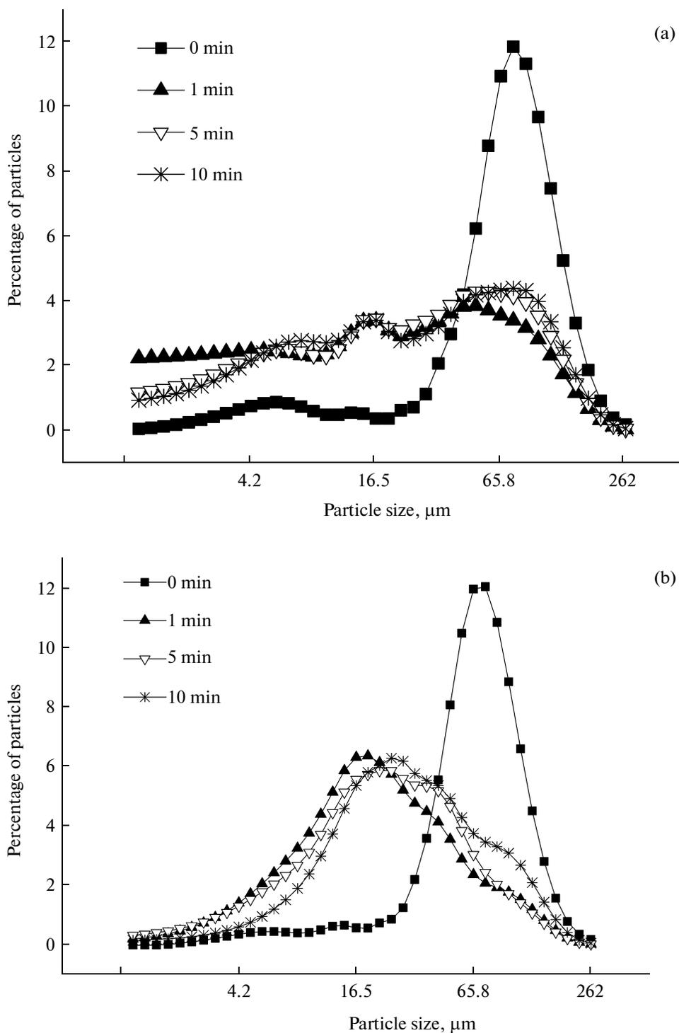
**Fig. 7.** Particle size distributions of the (a) unactivated and mechanically activated aluminum hydroxide and (b) lithium aluminate synthesized from the aluminum hydroxide.
