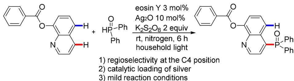
A simple and efficient protocol for the C4-H phosphonation of 8-hydroxyquinoline derivatives was developed under photoredox/silver(I) cocatalysis system
