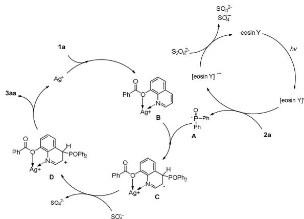
**Scheme 5.** Proposed mechanism of the phosphonation reactions
