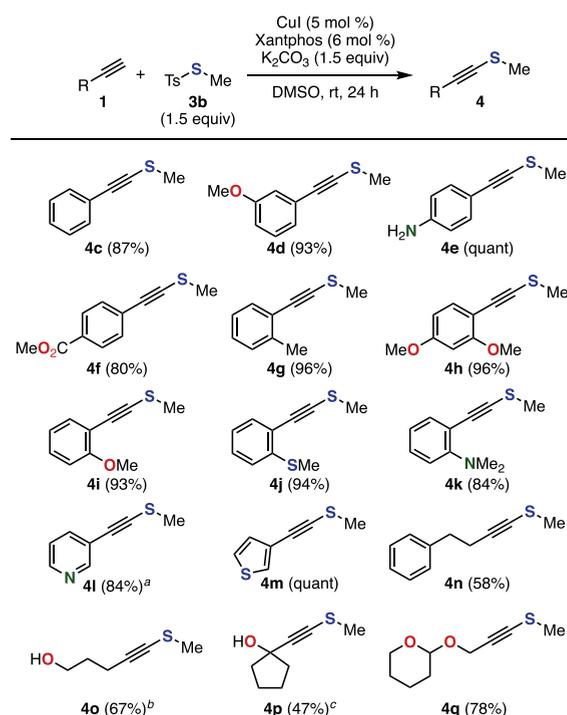
**Figure 2.** Thiolations of various terminal alkynes with S-methyl thiosulfonate **3b**. <sup>a</sup>CuI (10 mol %) and Xantphos (12 mol %) were used. <sup>b</sup>The reaction was performed using 3.0 equiv of **3b** at 100 °C for 1 h. <sup>c</sup>The reaction was performed using 3.0 equiv of **3b** at 50 °C for 12 h.
