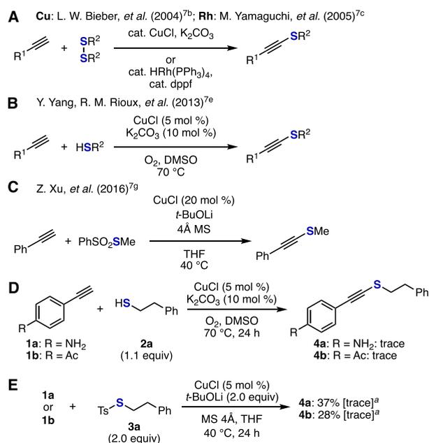
**Figure 1.** Reported methods for catalytic formation of alkynyl sulfides (A–C) and our attempts to synthesize alkynyl sulfides **4** by these methods (D and E). <sup>a</sup>K<sub>2</sub>CO<sub>3</sub> (2.0 equiv) was used instead of *t*-BuOLi. Yields were determined by HPLC.
