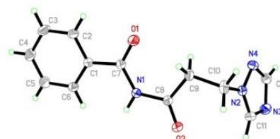
X-ray crystal structure of **2ab** showing the atom-labelling scheme. Displacement ellipsoids are drawn at the 30% probability level and H atoms are represented by circles of arbitrary radii.
