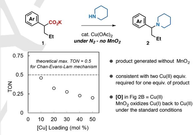
**Figure 7.** A) Use of alternative substrates support mechanism in which aryl acetate decarboxylation occurs prior to amination. B) Reaction stoichiometry in Cu(II) reflects a Chan-Evans-Lam type disproportionation redox pathway. Ar = 2-NO<sub>2</sub>-C<sub>6</sub>H<sub>4</sub> or 4-NO<sub>2</sub>-C<sub>6</sub>H<sub>4</sub>. See the SI for complete details.
