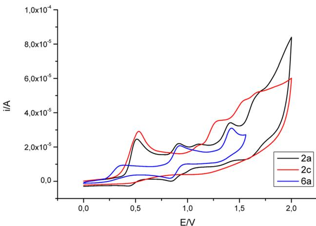
Figure 6. Cyclic voltammograms of **2a**, **2c**, and **6a** in CH<sub>3</sub>CN/0.1 M [NBu<sub>4</sub>]ClO<sub>4</sub> using Ag/AgCl 3 M as reference and a Pt wire counter electrode (scan rate 0.1 V/s).
