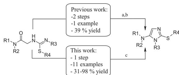
Figure 2. 2-Step synthesis of 5-amino-2-thioimidazole from *N*-acetamidoisothiourea precursor versus one step procedure using T3P. ((a) Lawesson's reagent, 1,2-dimethoxyethane, 20 °C, 16 h, (b) 4 N NaOH, 20 °C, (c) T3P, DIEA, EtOAc, microwave or classical heating.)
