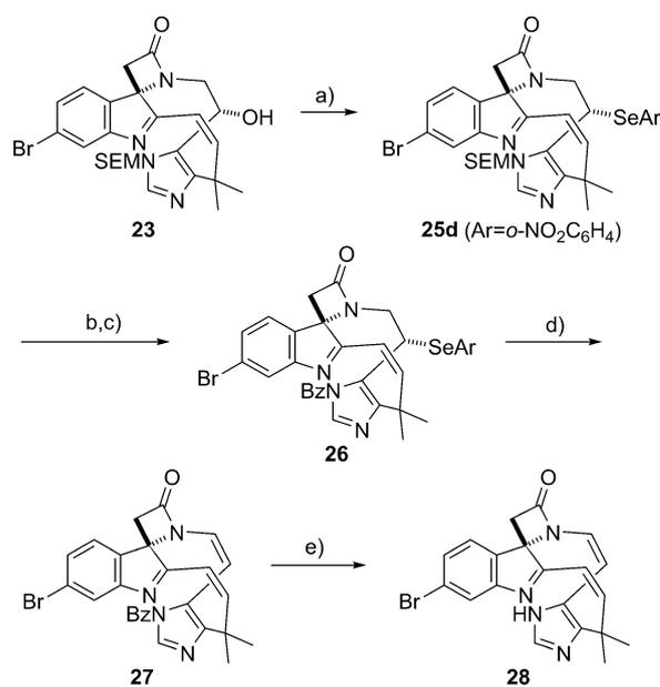
**Scheme 9.** a) *o*-NO<sub>2</sub>C<sub>6</sub>H<sub>4</sub>SeCN, *n*Bu<sub>3</sub>P, THF, RT, 62%; b) TfOH, CH<sub>2</sub>Cl<sub>2</sub>, –78 to 0°C; c) BzCl, Et<sub>3</sub>N, DMAP, CH<sub>2</sub>Cl<sub>2</sub>/THF (2:1), RT, 72% (2 steps); d) *m*CPBA, CH<sub>2</sub>Cl<sub>2</sub>, RT, 80%; e) Na<sub>2</sub>CO<sub>3</sub>, THF/H<sub>2</sub>O (2:1), RT, 63%. Bz = benzoyl, DMAP = 4-(dimethylamino)pyridine, *m*CPBA = *m*-chloroperbenzoic acid.
