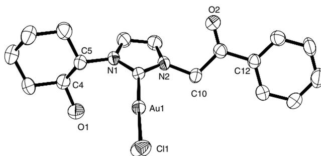
Fig. 3. ORTEP of **1c** with thermal ellipsoids drawn at 50% probability level. Selected bond lengths (Å) and angles (°): Au–C(1) 1.991(4), Au–Cl(1) 2.2921(11), N(1)–C(1) 1.344(5), N(2)–C(1) 1.356(5), C(1)–Au–Cl(1) 177.53(10), N(2)–C(1)–N(1) 105.9(3).
