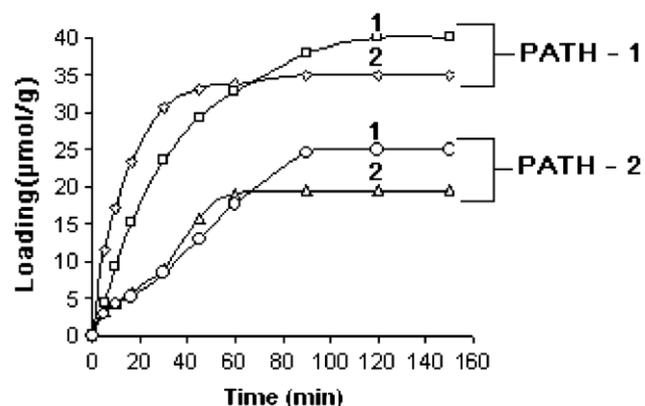
**Figure 1.** Time kinetics for aminoalkyl (1) and mercaptoalkyl (2) ligands, respectively, to know optimum time requirement for immobilizing biomolecules on the glass surface (CPG 500Å), via both the alternating paths.
