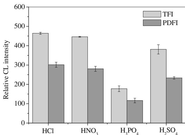
**Fig. 6** The effect of acids on CL intensity. Concentration: TFI, 0.1 mmol/L; PDFI, 0.1 mmol/L; acids, 0.5 mol/L;  $\text{KMnO}_4$ , 1 mmol/L. The error bars denote the standard deviation of the values with the three same determinations
