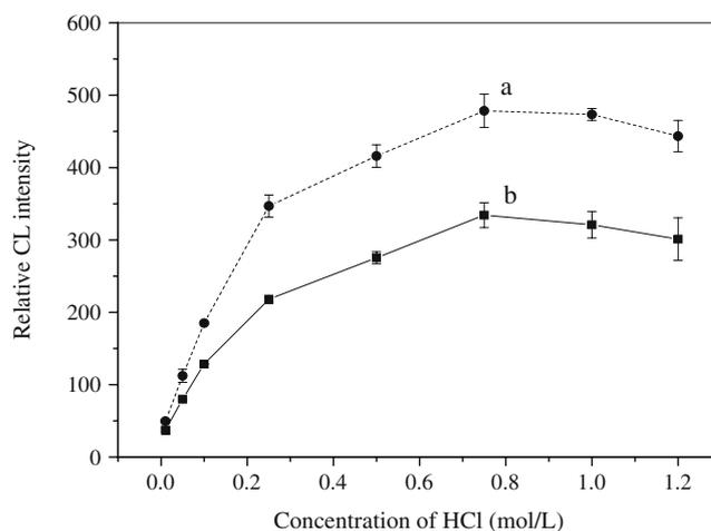
**Fig. 7** Influence of HCl concentration on the CL intensity. Concentration: **a** TFI, 0.1 mmol/L;  $\text{KMnO}_4$ , 1 mmol/L. **b** PDFI, 0.1 mmol/L;  $\text{KMnO}_4$ , 1 mmol/L. The error bars denote the standard deviation of the values with the three same determinations
