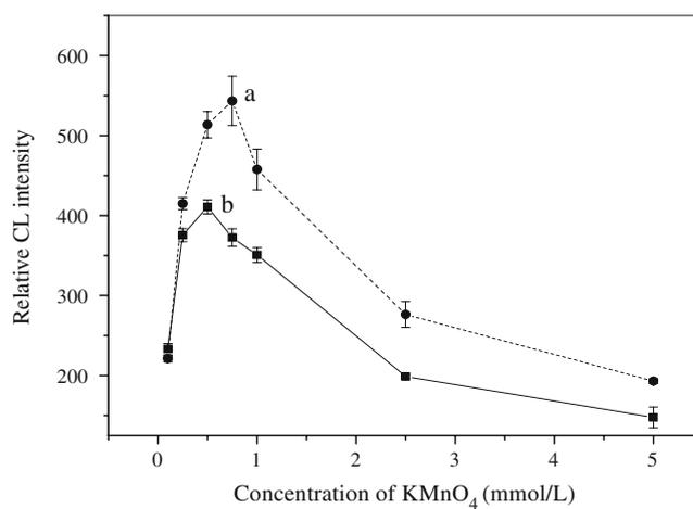
**Fig. 8** Influence of  $\text{KMnO}_4$  concentration on the CL intensity. Concentration: **a** TFI, 0.1 mmol/L;  $\text{HCl}$ , 0.75 mol/L. **b** PDFI, 0.1 mmol/L;  $\text{HCl}$ , 0.75 mol/L. The error bars denote the standard deviation of the values with the three same determinations
