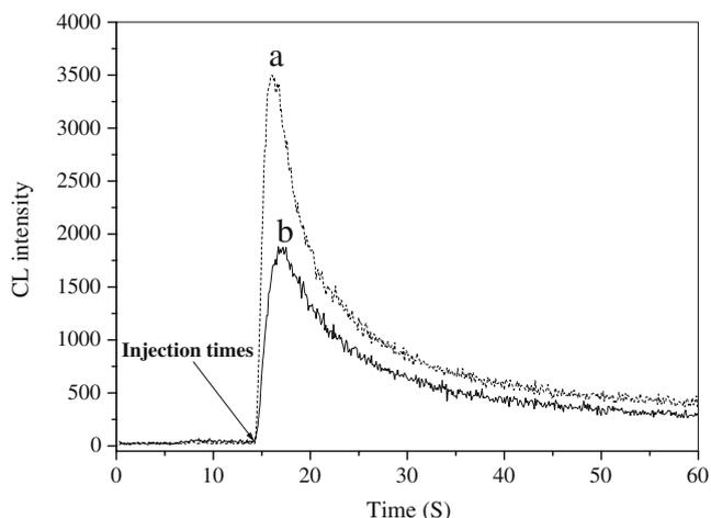
**Fig. 5** CL kinetic curves of TFI and PDFI. Concentration: **a** TFI, 0.1 mmol/L;  $\text{H}_2\text{SO}_4$ , 0.5 mol/L;  $\text{KMnO}_4$ , 1 mmol/L. **b** PDFI, 0.1 mmol/L;  $\text{H}_2\text{SO}_4$ , 0.5 mol/L;  $\text{KMnO}_4$ , 1 mmol/L
