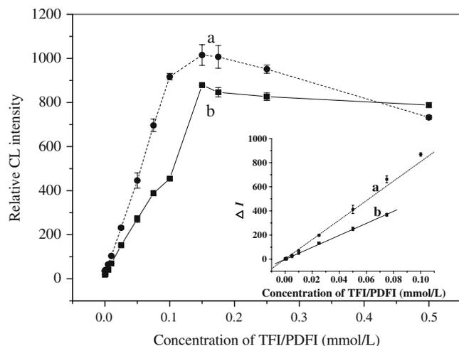
**Fig. 9** Influence of TFI/PDFI concentration on the CL intensity. The inset displays the linear relationship between  $\Delta I$  and the concentration of TFI/PDFI. **a** TFI-KMnO<sub>4</sub> system and **b** PDFI-KMnO<sub>4</sub> system. Concentration: **a** HCl, 0.75 mol/L; KMnO<sub>4</sub>, 0.75 mmol/L. **b** HCl, 0.75 mol/L; KMnO<sub>4</sub>, 0.5 mmol/L. The error bars denote the standard deviation of the values with the three same determinations
