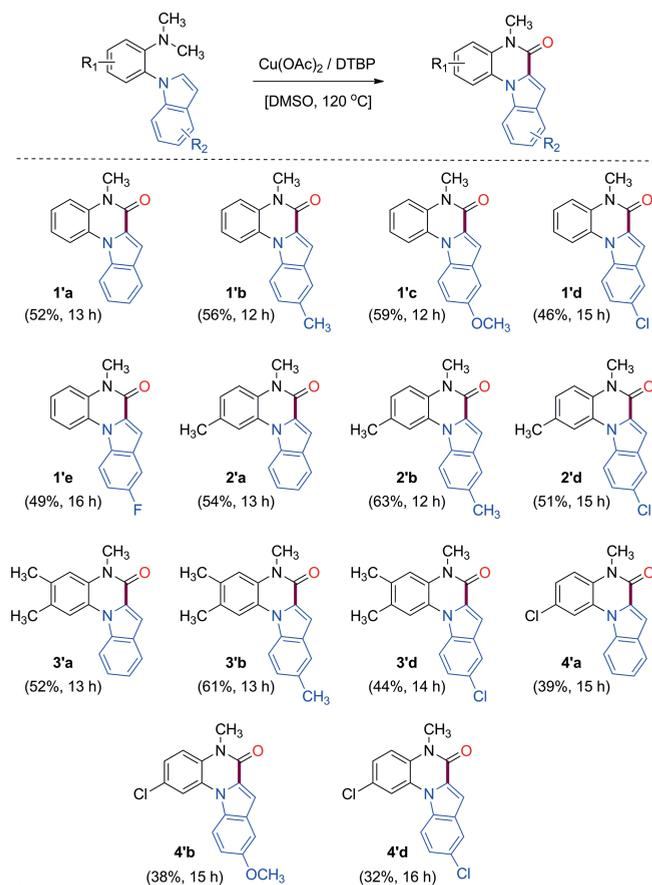
Scheme 2. Substrate scope for indoloquinoxalin-6-ones.<sup>[a,b]</sup> [a] Reaction conditions: *o*-indolyl-*N,N*-dimethylamine (0.25 mmol),  $\text{Cu}(\text{OAc})_2$  (0.025 mmol), and DTBP (1.5 mmol) in DMSO (1 mL) at 120 °C. [b] Yield of isolated pure product.
