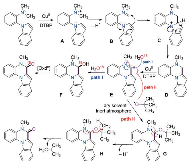
Scheme 4. Plausible mechanism for the formation of indoloquinoxalin-6-one.
