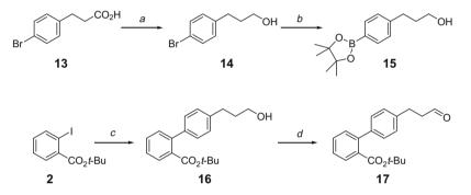
Scheme 2. Reagents and conditions: (a) LAH, ether, 0 °C to rt; (b) bis(pinacolate)diboron, Pd(dppf), KOAc, DMSO; (c) 15, Pd(dppf), Na<sub>2</sub>CO<sub>3</sub> (2 N),DMF, 85 °C; (d) TEMPO (cat.), trichloroisocyanuric acid, CH<sub>2</sub>Cl<sub>2</sub>, 0 °C to rt.
