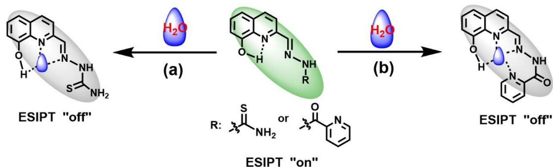
**Scheme 2.** Proposed detection mechanisms of HQCT (a) and HQPH (b) toward H<sub>2</sub>O.
