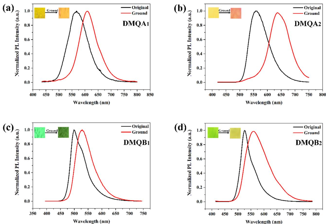
Fig. 4. PL spectra in solid states of the original and grounded samples. (a)  $DMQA_1$ ; (b)  $DMQA_2$ ; (c)  $DMQB_1$  and (d)  $DMQB_2$ .
