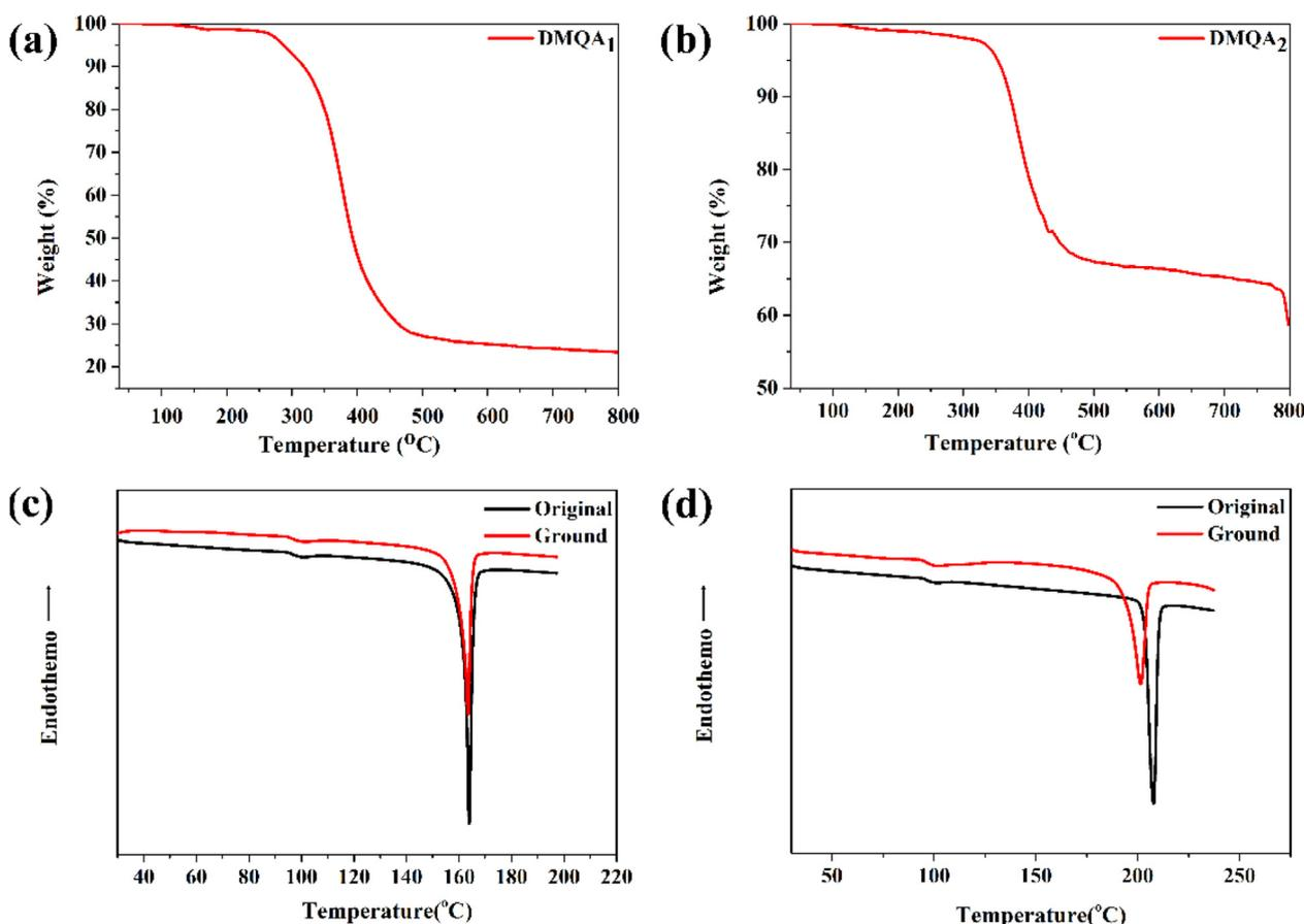
Fig. 8. TGA curves of (a) DMQA<sub>1</sub> and (b) DMQA<sub>2</sub>; DSC curves of (C) DMQA<sub>1</sub> and (D) DMQA<sub>2</sub>.
