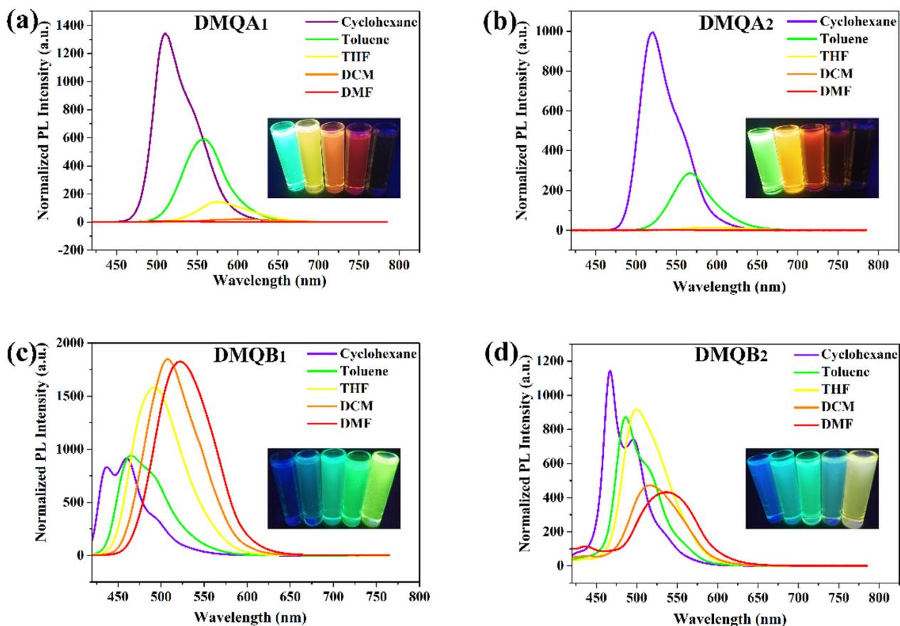
Fig. 1. The PL spectra in solvents with different polarity of (a)  $DMQA_1$  (b)  $DMQA_2$  (c)  $DMQB_1$  (d)  $DMQB_2$ . The concentration of the solutions is  $1.0 \times 10^{-4} \text{ mol L}^{-1}$ .
