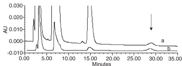
Fig. 4. Chromatograms of the reaction of enalaprilat with the MPO/H<sub>2</sub>O<sub>2</sub>/Cl<sup>-</sup> system and HOCl in the following conditions; a: pH 7.4 PBS buffer (NaCl 300 mM and PO<sub>4</sub><sup>3-</sup> 10 mM), enalaprilat (600 μM), MPO (51 nM), H<sub>2</sub>O<sub>2</sub> (100 μM); b: pH 7.4 PBS buffer, enalaprilat (60 μM) and HOCl (60 μM). The peak marked with ↓ corresponds to the product of oxidation by the both systems.
