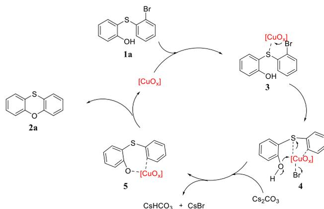
**Scheme 2.** Proposed mechanism for synthesis of phenoxathiins.
