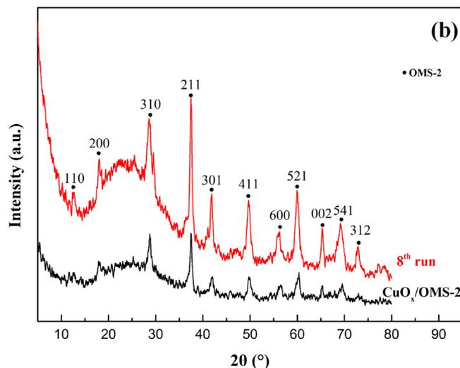
**Fig. 2.** (a) TEM and (b) XRD of 8th used CuO<sub>x</sub>/OMS-2 catalyst.
