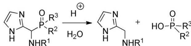
**Scheme 3.** Decomposition of imidazole-2-yl-(amino)methylphosphorous derivatives **3, 4** and **6** in the presence of a strong mineral acid.
