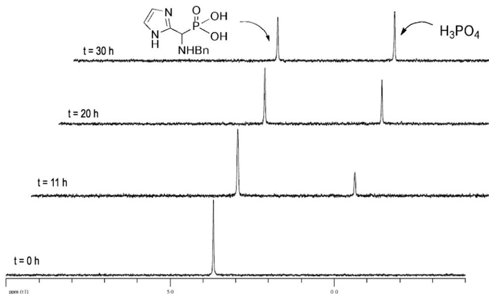
Fig. 2. Kinetic experiment of the cleavage of **6b** in 1.0 M  $\text{H}_2\text{SO}_4$  monitored by  $^{31}\text{P}$  NMR.
