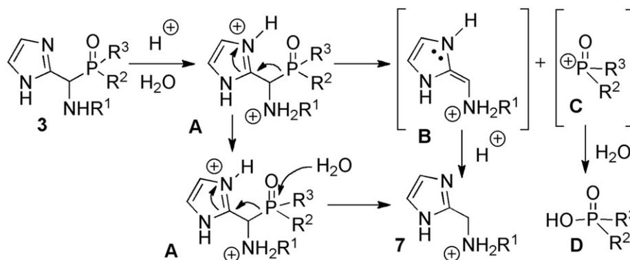
Scheme 4. Possible mechanistic pathways of the cleavage.
