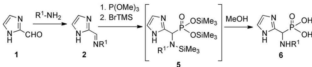
**Scheme 2.** Preparation of imidazol-2-yl-(amino)methylphosphonic acids **6**.
