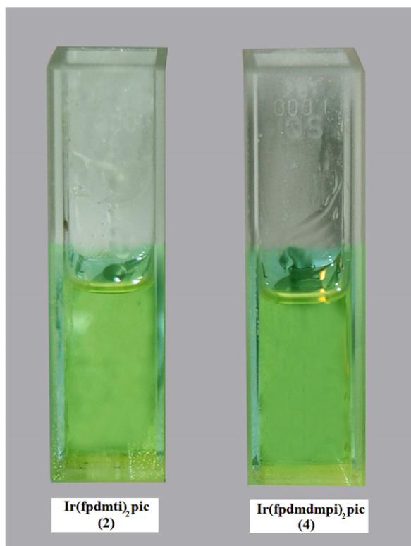
Fig. 13. Solution color of the photoluminescence for complexes 2 and 4 in  $\text{CH}_2\text{Cl}_2$ .
