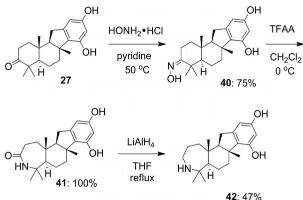
Scheme 5. Synthesis of A ring functionalized analogs of pelorol.
