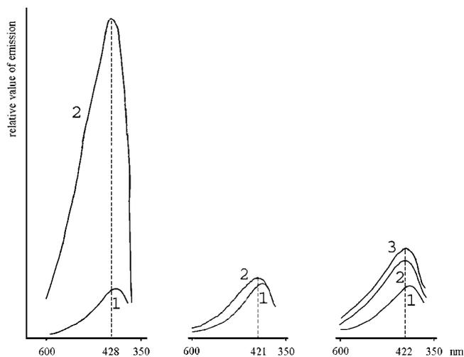
Figure 3. Fluorescence spectra (methanol,  $10^{-4}$  M): 1 – background; left: 2 – methoxy-substituted triazine **3d**; center: 2 – triazine **3a**; right: 2 – oxazole **2a**, 3 – oxazole **2a** after addition of hydrazine hydrate (3 equiv.)
