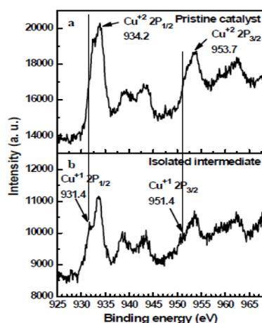
**Figure 2.** High resolution XPS spectra of Cu 2p in ionic liquid supported Cu(II) catalyst before and after the reaction.
