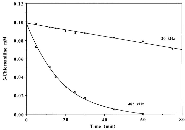
Fig. 3. Kinetics of ultrasonic transformation of 3-chloroaniline at 20 and 482 kHz in air-equilibrated solution (100 ml).
