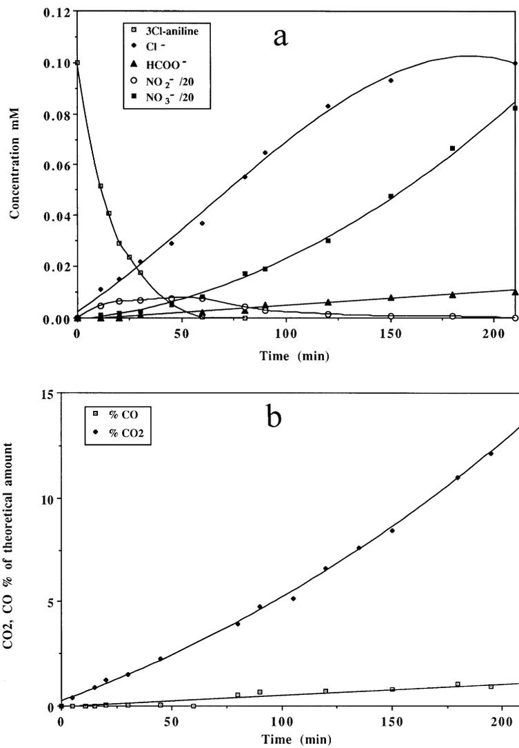
Fig. 4. Kinetics of formation of the main sonoproducts of 3-chloroaniline at 482 kHz in air-equilibrated solution (100 ml). (a) Organic and ionic products; (b) carbon monoxide and dioxide.
