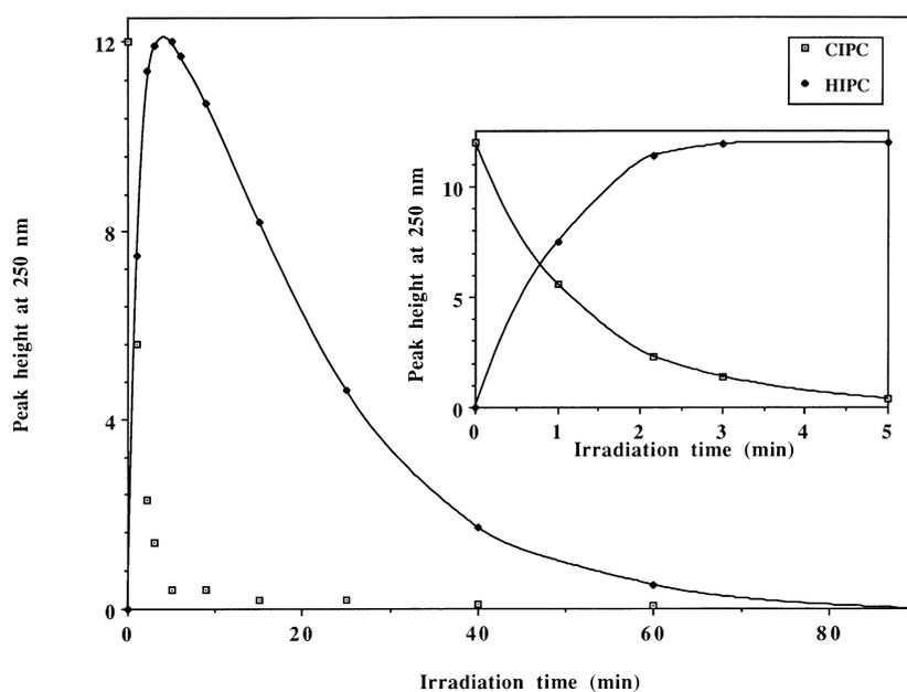
Fig. 7. Kinetics of phototransformation of a solution of chlorpropham  $1.45 \times 10^{-4}$  M, irradiated at 254 nm (detection at 250 nm, photon rate received in 25 ml  $\approx 2 \times 10^{-6}$  Einstein  $s^{-1}$ ).
