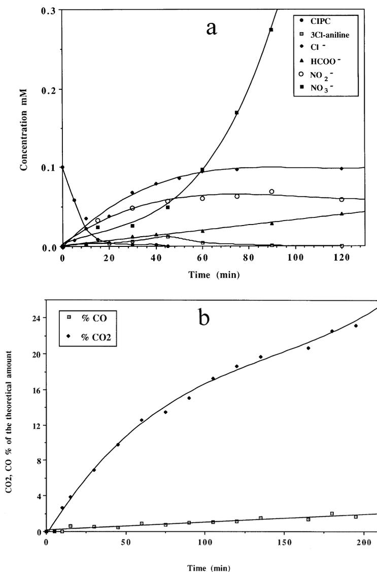
Fig. 2. Kinetics of formation of the main sonoproducts of chlorpropham at 482 kHz in air-equilibrated solution (100 ml, 0.1 mM). (a) Organic and ionic products; (b) carbon monoxide and dioxide.
