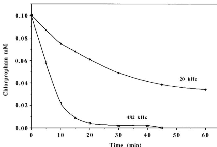
Fig. 1. Kinetics of ultrasonic transformation of chlorpropham (CIPC) at 20 and 482 kHz in air-equilibrated solution (100 ml).
