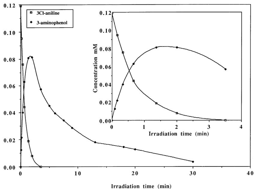
Fig. 8. Kinetics of transformation of 3-chloroaniline  $1.2 \times 10^{-4}$  M and formation of the main photoproducts by irradiation at 254 nm (detection at 270 nm, photon rate received in 25 ml  $1.8 \times 10^{-6}$  Einstein  $s^{-1}$ ).
