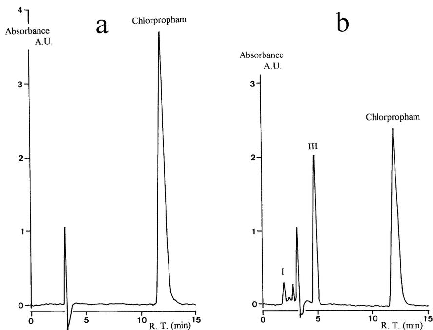
Fig. 6. HPLC chromatogram of an unbuffered air-saturated solution of chlorpropham  $1.7 \times 10^{-4}$  M. (a) Non-irradiated; (b) irradiated during 1 min at 254 nm (photon rate  $1.6 \times 10^{-7}$  Einstein  $s^{-1}$  in 10 ml, conversion 36%) eluent MeOH/H<sub>2</sub>O, 68/32, detection 270 nm.
