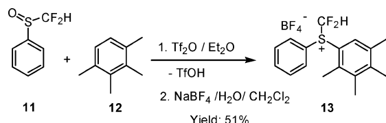
Scheme 2. Preparation of S -Difluoromethyl- S -phenyl-2,3,4,5-tetramethylphenylsulfonium Tetrafluoroborate ( 13 )
