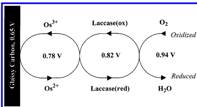
centers of the electron and ion-conducting redox polymer to  $\text{Os}^{3+}$ , and the redox polymer is electroreduced at the carbon surface at a potential near 0.65 V.
