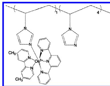
**Figure 1.** Structure of the laccase wiring redox polymer.
