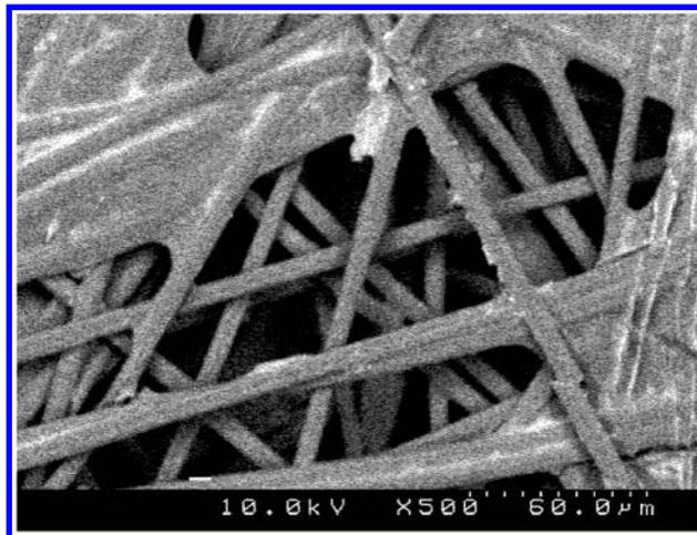
**Figure 2.** SEM (electron backscattering mode) of the composite 350  $\mu\text{m}$  thick carbon cloth cathode loaded with 0.78  $\text{mg}/\text{cm}^2$  “wired” laccase (45 wt % laccase, 49 wt % redox polymer, 6 wt % PEGDGE). The lighter areas are coated with more heavy atoms (osmium).
