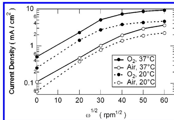
**Figure 4.** Dependence of the current density of O<sub>2</sub> electroreduction at 0.62 V (NHE) on the square root of the angular velocity of the rotating electrode. Conditions as in Figure 3b.
