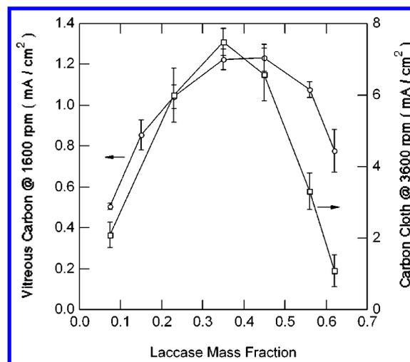
**Figure 5.** Dependence of the O<sub>2</sub> electroreduction current density at 0.62 V (NHE) on the laccase loading. Total loading was fixed at 0.78 mg/cm<sup>2</sup> and PEGDGE constituted 6 wt % of the total mass. Conditions as in Figure 3b.
