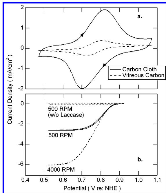
**Figure 3.** (a) Cyclic voltammograms (50 mV/s sweep rate, 500 rpm) of the vitreous carbon and the composite carbon cloth electrodes under argon. (b) Potential-dependence of the O<sub>2</sub> electroreduction current density at 1 mV/s sweep rate at 1 atm O<sub>2</sub> pressure. Loading as in Figure 2, 0.2 M citrate buffer, pH 5, 37 °C. Current densities were based on the projected area of the 4-mm carbon cloth disk (0.13 cm<sup>2</sup>).
