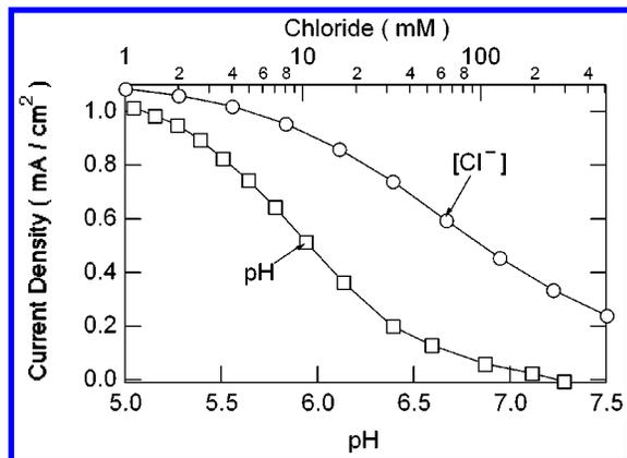
**Figure 6.** Dependence of the current density of the noncomposite (polished and catalyst coated) vitreous carbon electrodes on pH and on the chloride ion concentration. 0.62 V (NHE), 900 rpm. Conditions as in Figure 3b.
