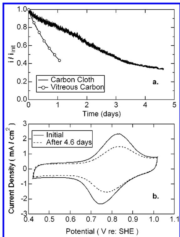
**Figure 7.** Operational stability of the "wired" laccase electrode. (a) Time-dependence of the current density of carbon-cloth composite and of the vitreous carbon noncomposite electrodes poised at 0.62 V (NHE). (b) The change in the cyclic voltammograms of the carbon cloth composite electrode after 4.6 days of operation. Scan rate 50 mV/s. The composition, loading and conditions were as in Figure 3b.
