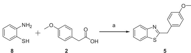
**Scheme 3.** Synthesis of benzothiazole **5**. Reagents and conditions: (a) boric acid, xylene, reflux, 16 h, 48%.
