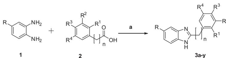
**Scheme 1.** Synthesis of benzimidazole derivatives **3a–y** (substituents are listed in Table 1). Reagents and conditions: (a) boric acid, xylene, reflux, 12–16 h, 45–90%.
