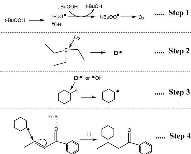
**Scheme 1** Some inferred steps in the overall synthesis of 3-cyclohexyl-1-phenyl-1-butanone (CPB).
